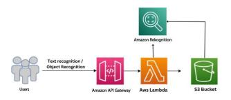
Fig. 5. AWS Rekognition block diagaram
